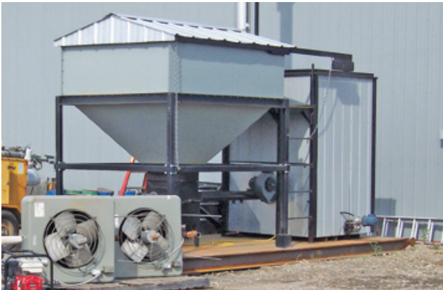
Portable Skid-Mounted Boiler for Easy Setup
